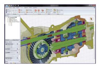
SpaceClaim's Pull, Move, Fill, and Combine tools let you work in 3D and cross sections to create new design concepts using existing data from any CAD system.
